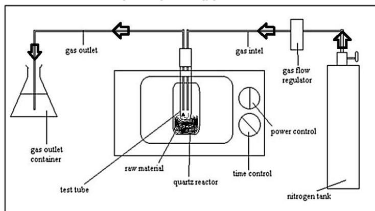
Figure 3.1. Microwave Torrefaction Apparatus Schematic
