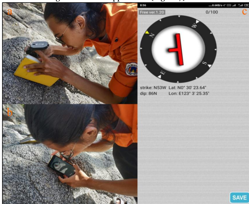
Figure 7. Structural geological data collection. a) Data collection using a compass, b) Data collection using mobile learning, c) The results of data measurement on the mobile application.
