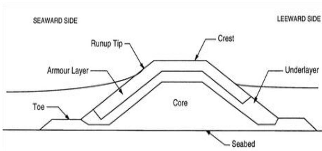
**Figure 2.** Cross section of a typical rubble mound breakwater.
