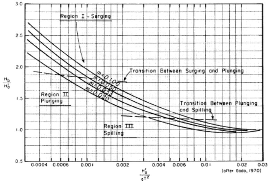
**Figure 3.** Breaker wave height index versus deepwater water steepness (Shore Protection Manual, 1984)
