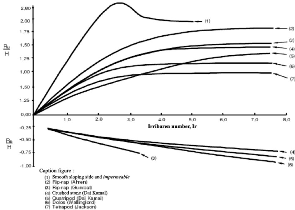
**Figure 5. Wave run up** (Shore Protection Manual, 1984)
