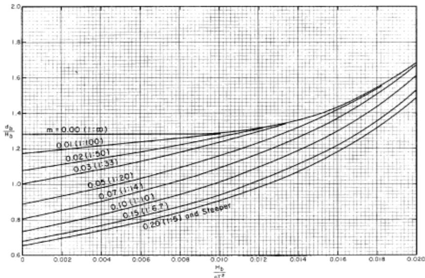
**Figure 4.** Water depth at the location of breaking wave (Shore Protection Manual, 1984)
